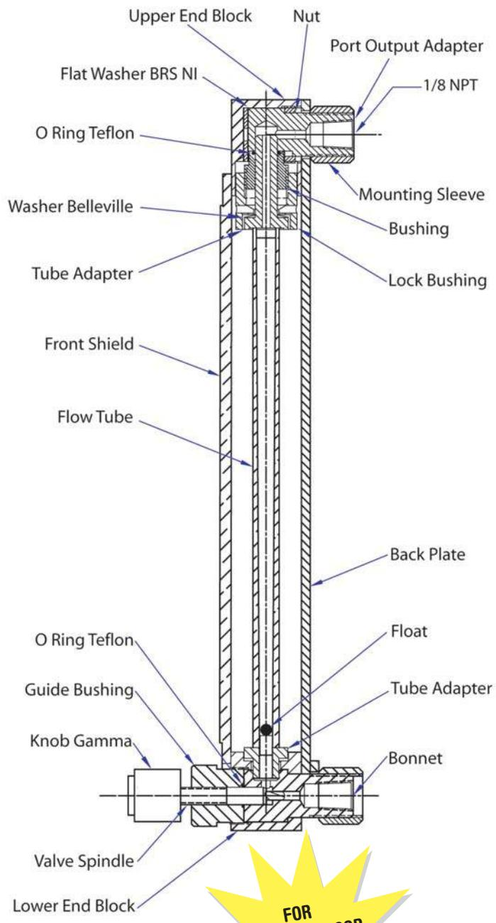
Panel mounting is convertible to bench mounting through the use of an optional acrylic tripod base with spirit leveler (catalog No. TP1).
