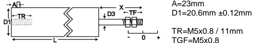
Our DCTH captive guided displacement transducer has bearings to guide the armature inside the measurement sensor. Our DCTH captive LVDTs are for position measurement applications where guidance may be poor and end bearings may be required.
