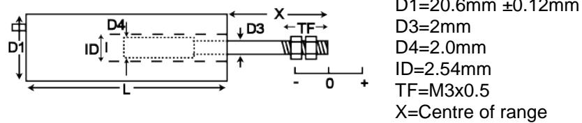
On our DCTH unguided LVDTs the armature assembly is a separate component, to make a measurement the user must guide the armature inside the body without touching the sides. Our DCTH unguided position measurement transducers are appropriate where external guidance is available and give truly non-contact operation
