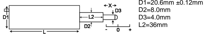
Our DCTH spring displacement transducer has bearings to guide the armature inside the measurement sensor and a spring which pushes the armature to the fully out position. Our DCTH spring return LVDTs are appropriate where it is not possible to connect the transducer armature to the moving component being measured.
