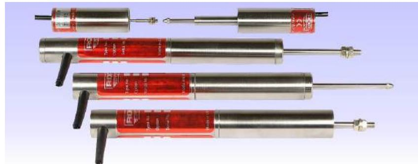
These transducers are for displacement / position measurement. They make an accurate position measurement of the movement of the armature (the sliding part) relative to the body of the displacement transducer.
