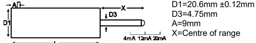
Our DCC spring displacement transducer has bearings to guide the armature inside the measurement sensor and a spring which pushes the armature to the fully out position. Our DCC spring return LVDTs are appropriate where it is not possible to connect the transducer armature to the moving component being measured.
