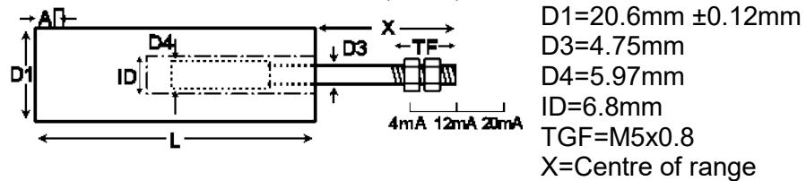
On our DCC unguided LVDTs the armature assembly is a separate component, to make a measurement the user must guide the armature inside the body without touching the sides. Our DCC unguided position measurement transducers are appropriate where external guidance is available and give truly non-contact operation
