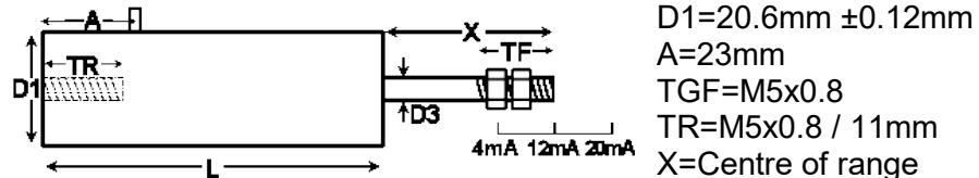
Our DCC captive guided displacement transducer has bearings to guide the armature inside the measurement sensor. Our DCC captive LVDTs are for position measurement applications where guidance may be poor and end bearings may be required.
