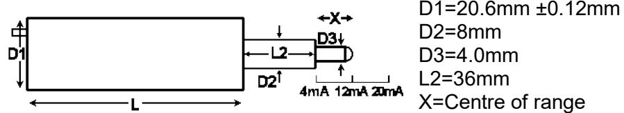
DCC025A to DCC150A - Side (radial) exit cable
