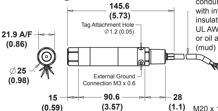
M20 x 1.5 or 1/2 NPT conduit connection with integrated TPE insulated and jacketed UL AWM 20237 or oil and drilling fluid (mud) resistant cable.
