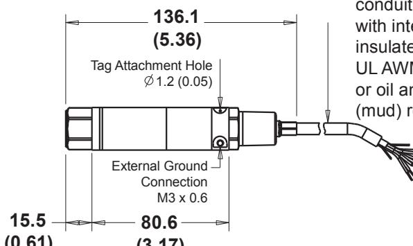
M20 x 1.5 or 1/2 NPT conduit connection with integrated TPE insulated and jacketed UL AWM 20237 or oil and drilling fluid (mud) resistant cable.
