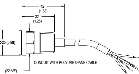
CONDUIT WITH POLYURETHANE CABLE
